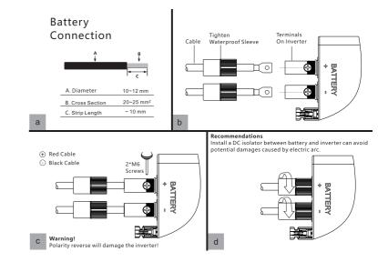
Step 2: Install the battery power connector.
