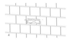
Step2: Install the inverter on the wall-mounting bracket and lock the inverter using the security screws.
