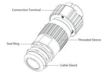
a) Lead the AC cable though cable gland, seal ring and threaded sleeve, and fully insert the conductors to corresponding terminals on connection terminal and tighten the screws.
